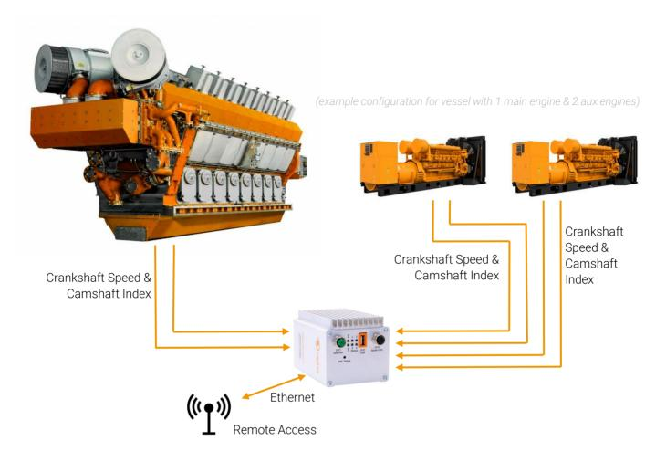
smartAlpha™ is non-intrusive and easy to retrofit. Existing speed sensor signals can often be used.
