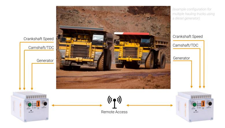
smartAlpha™ is non-intrusive and easy to retrofit. Existing speed sensor signals can often be used.
